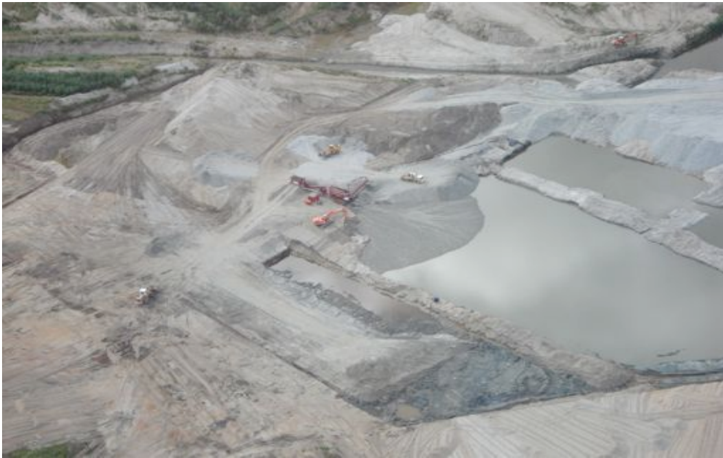
A large placer operation on lower Dominion Creek, Klondike District. Mined out areas are used to accept fresh tailings and to act as settling ponds. A methodical approach to mining is required to successfully mine these low-grade high volume placers.
